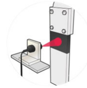
FIGURE 22. Thermal monitoring inside the switchgear panels and control panels from [166].
